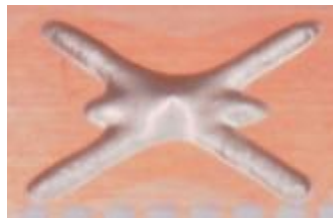
Dispense Patterns Visible solvent bleed out
