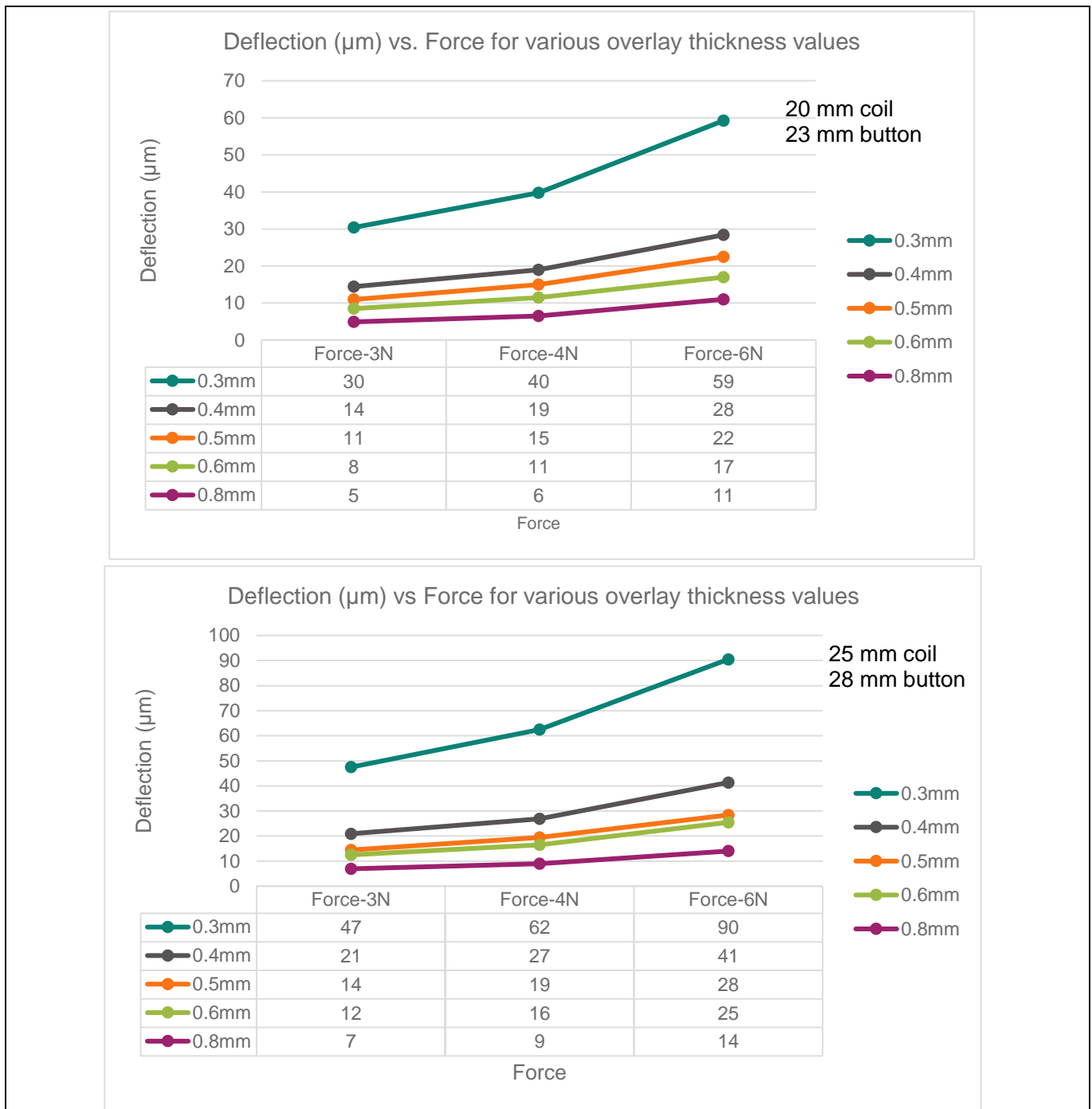
Figure 43 Deflection values ( in µm) for different overlay thickness values and button (coil) sizes
