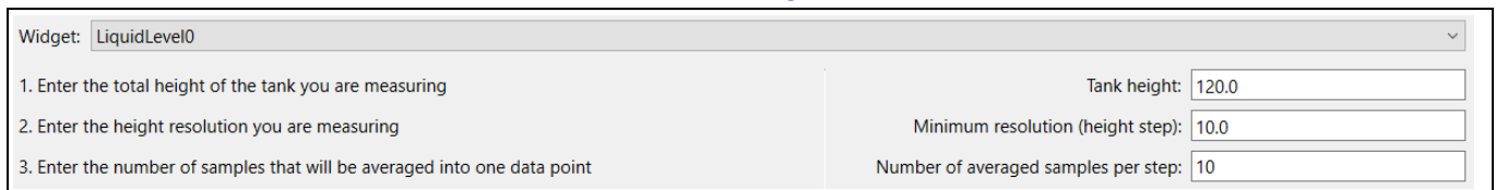
Figure 8 Liquid-level measurement parameters
