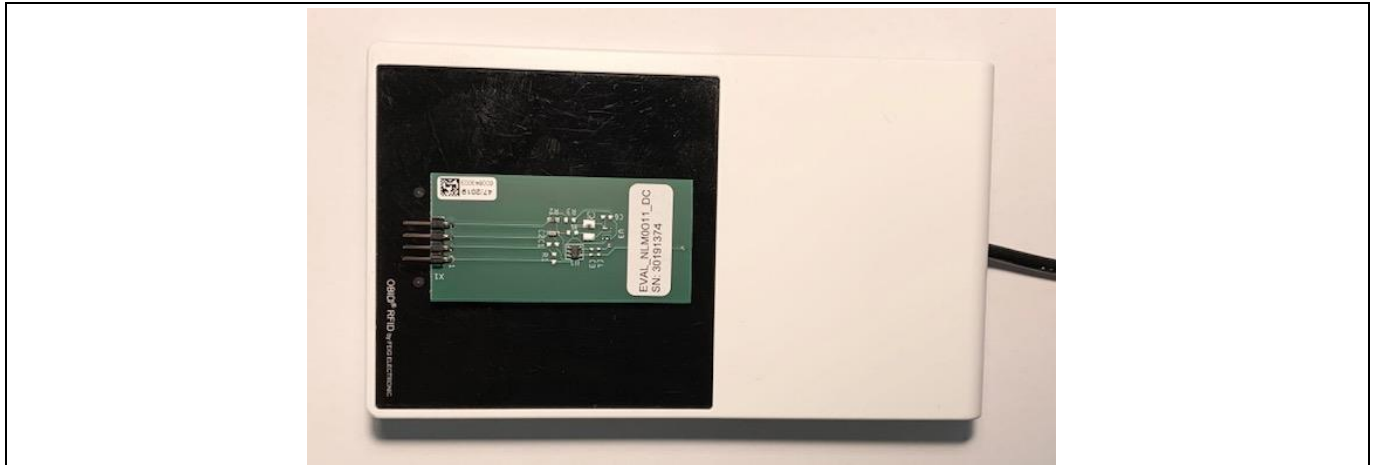
Figure 15 Board “DK_NLM_02” placed on CPR30 reader
