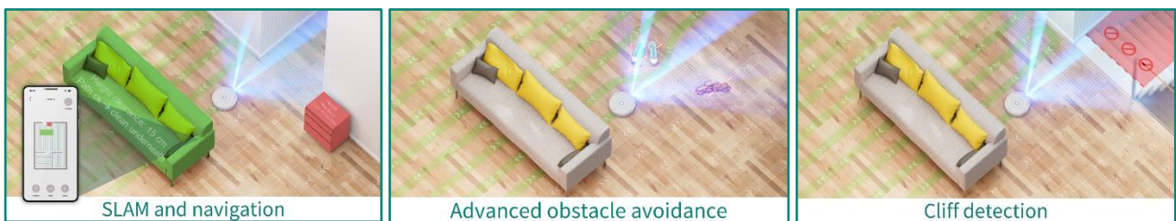
Figure 1 Primary robotic use cases addressed by hToF: SLAM and navigation, advanced obstacle avoidance, and cliff detection
