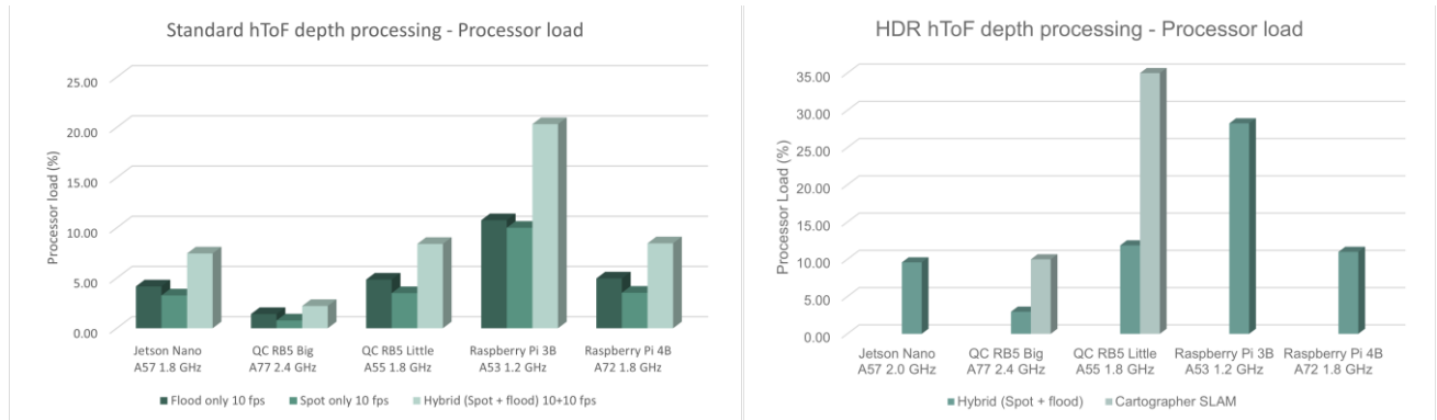
Figure 11 Processor load for standard hToF depth processing (left) and HDR hToF depth processing (right)
