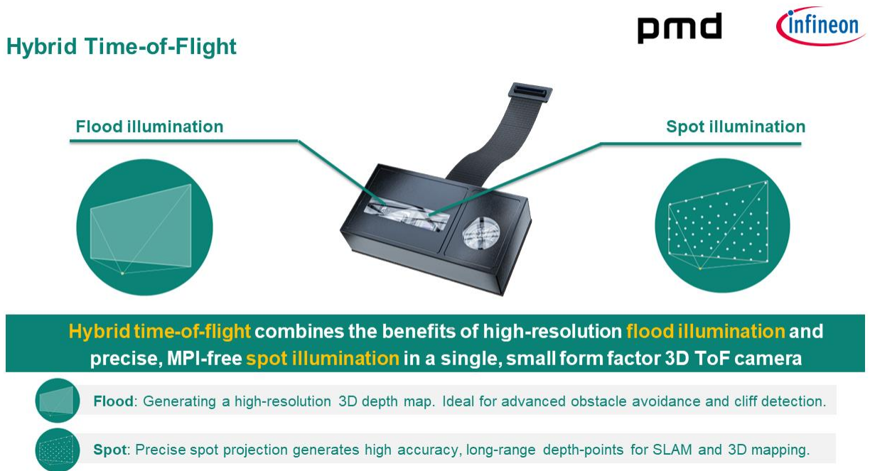
Figure 2 Overview of a hybrid Time-of-Flight module’s characteristics, the spot and flood types of illumination, and its advantages for robotics that support SLAM, advanced obstacle avoidance, and cliff detection
