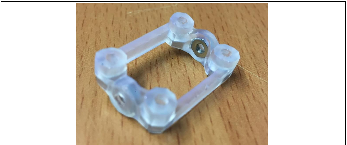
Figure 9 Camera mounting assembled with nuts
