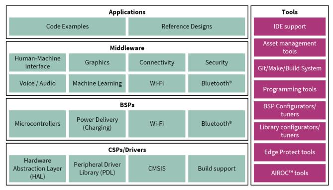
One part of the ModusToolbox<sup>™</sup> ecosystem is run-time software that helps you rapidly develop applications using Infineon BSPs.
