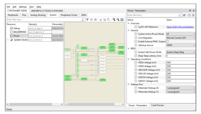
There are settings for the PSoC<sup>™</sup> 6 MCU and the connectivity combo device. For more details about how to configure low power, refer to the LPA Guide here:
