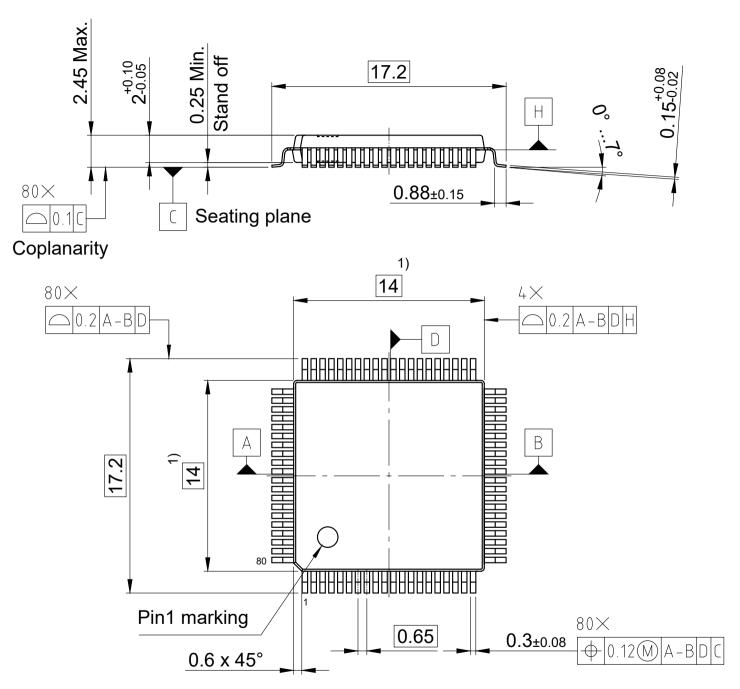
1) Does not include plastic or metal protrusion of 0.25 max. per side All dimensions are in units mm
