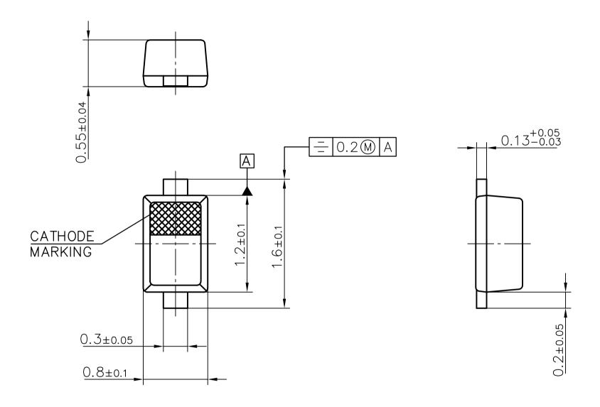
ALL DIMENSIONS ARE IN UNITS MM THE DRAWING IS IN COMPLIANCE WITH ISO 128 & PROJECTION METHOD 1 [--]
