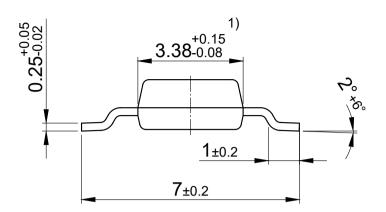
1) All dimensions refer to JEDEC standard TO261-AA do not include mold flash or protrusions, body length including mold protrusions shall not exceed 6.7mm.
