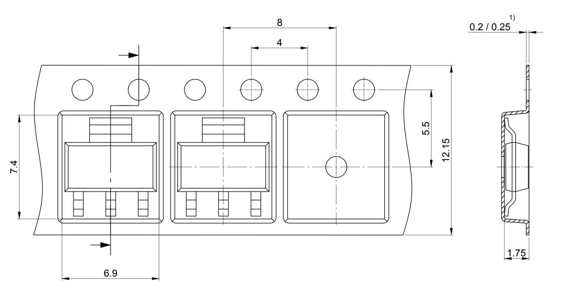
1) Thickness value can be either 0.2mm or 0.25mm
