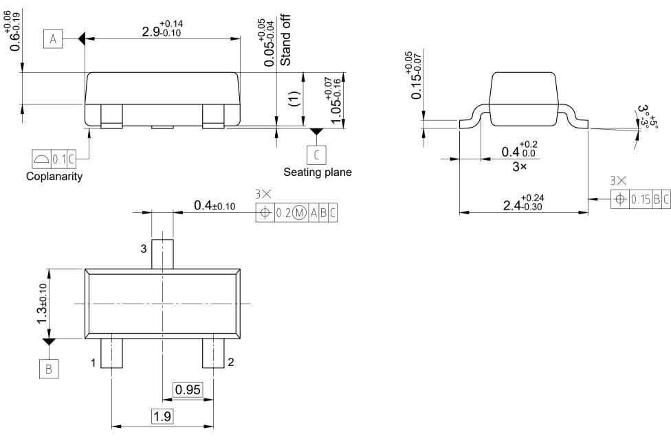
Dimensions does not include mold protrusions or interlead flash. Mold protrusion or interlead flash shall not exceed 0.25 per side. All dimensions are in units mm The drawing is in compliance with ISO 128-30, Projection Method 1 [
