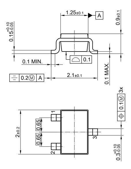
MOLD FLASH, PROTRUSION OR GATE BURRS OF 0.2 MM MAXIMUM PER SIDE ARE NOT INCLUDED ALL DIMENSIONS ARE IN UNITS MM THE DRAWING IS IN COMPLIANCE WITH ISO 128 & PROJECTION METHOD 1 [  $\bigcirc$  ]
