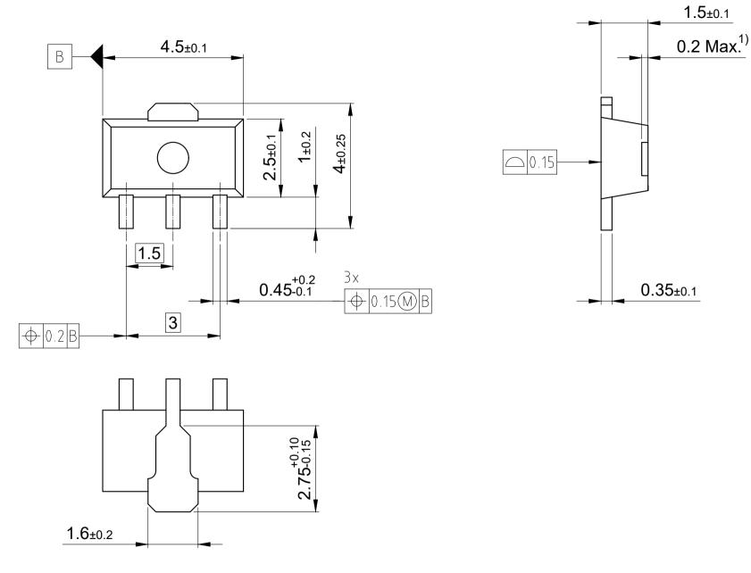
1) Ejector pin marking possible
