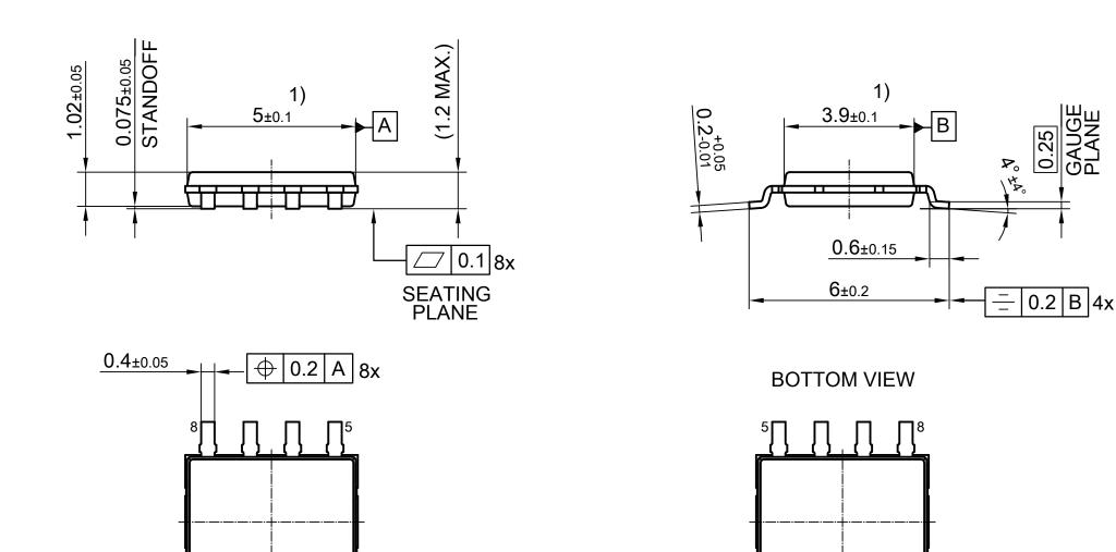
1) OUTER DIMENSION DOES NOT INCLUDE PROTUSION OR INTRUSION OF 0.15 PER SIDE ALL DIMENSIONS ARE IN UNITS MM THE DRAWING IS IN COMPLIANCE WITH ISO 128 & PROJECTION METHOD 1 [  $\rightleftharpoons$  ]
