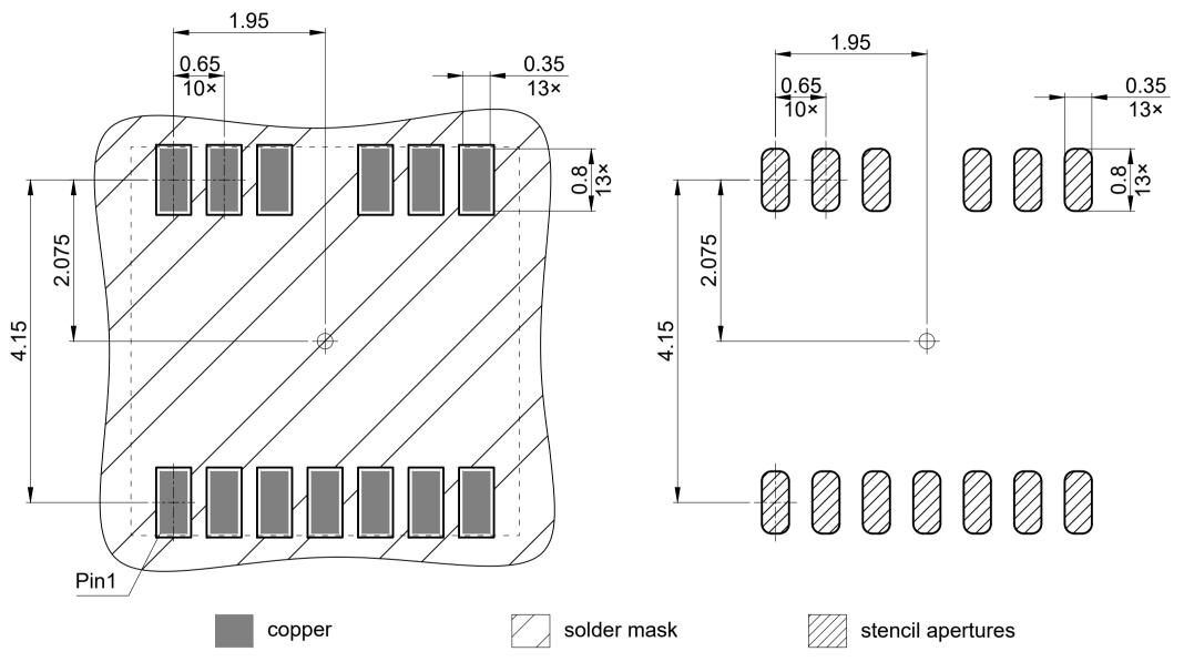
All pads are non-solder mask defined All undimensioned radii are 0.125 All dimensions are in units mm
