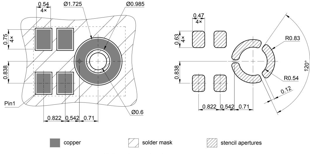
All dimensions are in units mm All pads are non-solder mask defined All undimensioned radii are 0.1
