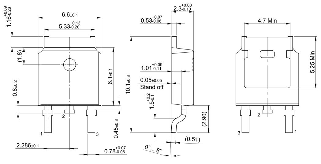
All dimensions refer to JEDEC standard TO-252 AA and do not include mold flash or protrusions All dimensions are in units mm
