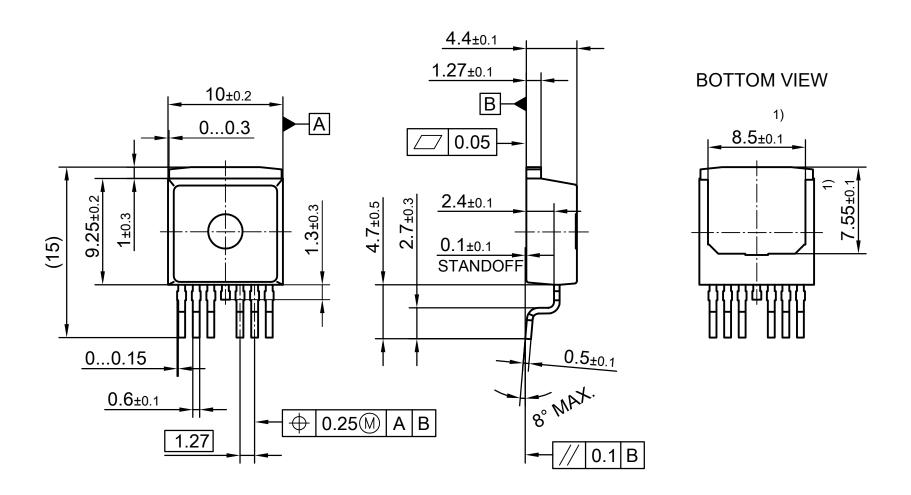
1) TYPICAL METAL SURFACE MIN. X = 7.25, Y = 6.9 ALL METAL SURFACES: TIN PLATED, EXCEPT AREA OF CUT ALL DIMENSIONS ARE IN UNITS MM THE DRAWING IS IN COMPLIANCE WITH ISO 128 & PROJECTION METHOD 1 [  $\bigcirc \bigcirc$  ]
