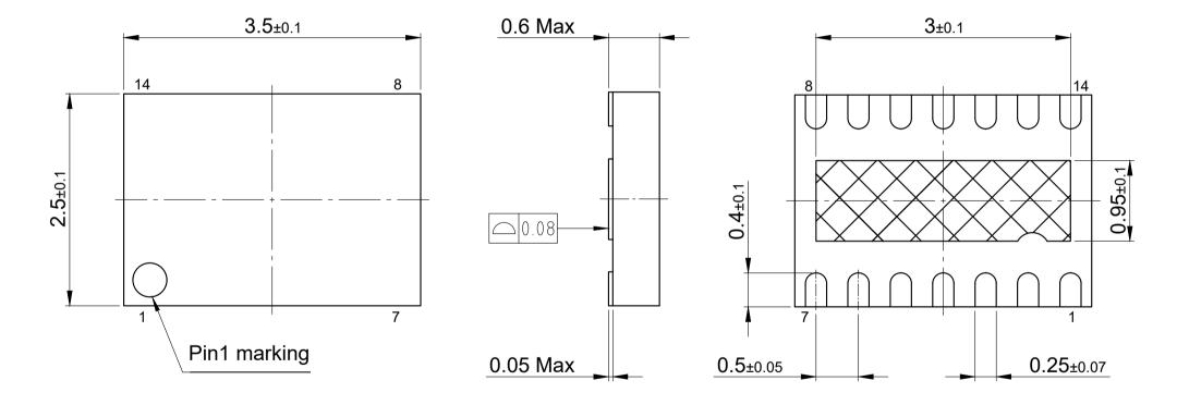
Hatch area is solderable exposed metal.
