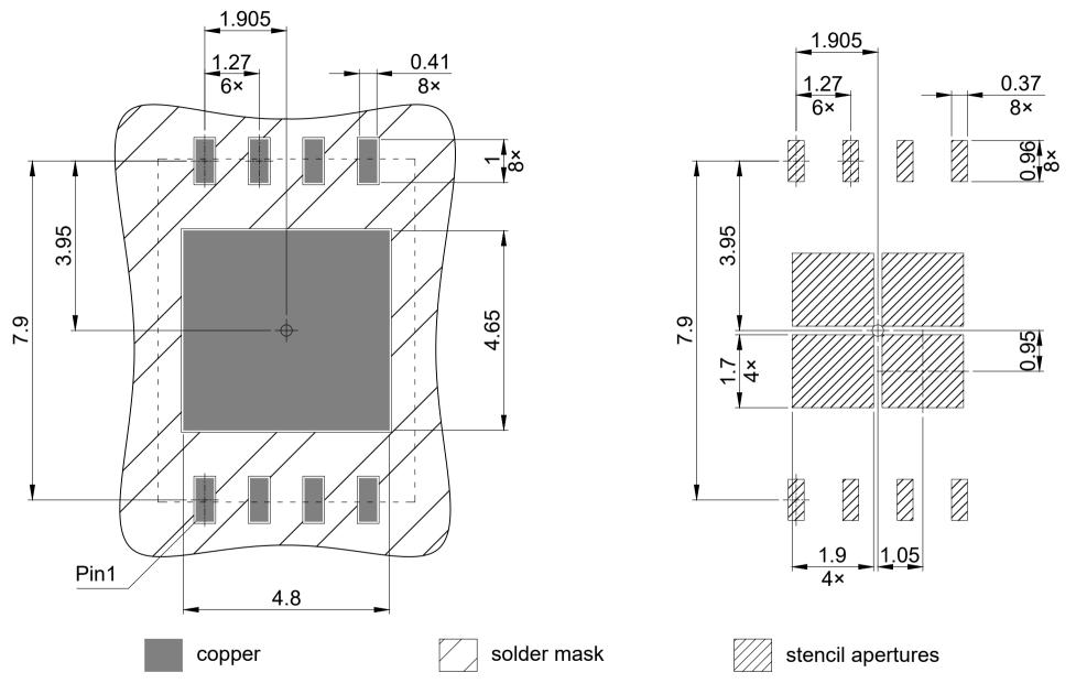
All dimensions are in units mm Based on stencil thickness 0.13 mm All pads are non-solder mask defined
