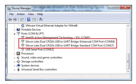
Open UART properties. Expand Ports (COM & LPT), right-click on Silicon Labs Dual CP210x USB to UART Bridge: Enhanced COM Port (COM17), and then click Properties. CPM17 will be connected to the PS UART0 and COM18 will be connected to the PS UART1. In this tutorial, we will be using the PS UART0 as STDOUT and STDIN. • In the properties window, select the Port Settings tab; verify the settings match the values shown in the following figure. Click on the **Advanced** button to continue.
